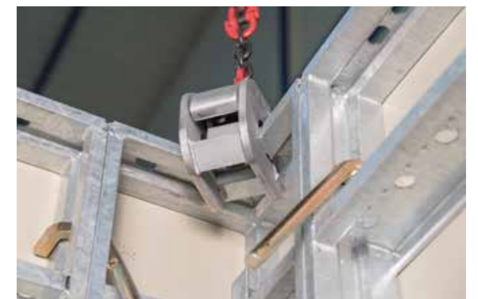
▶ With the transport hook, the corners can also be moved in a centrally attached position.
