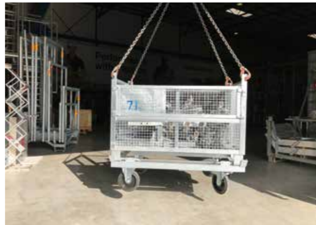
► The grid box enables the storage of connecting elements, anchor nuts, etc. It can be attached to the carriage and moved by crane. Simple handling saves considerable crane time – a clear improvement for storage and logistics.
