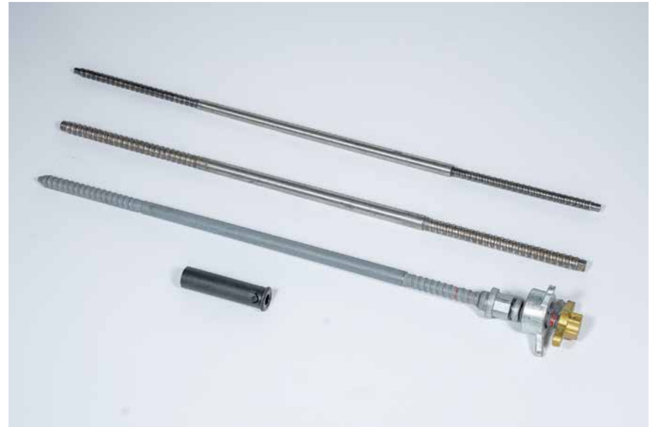
▶Flexible: Various tie systems can be used. Here, the efficient PLATINUM 100 tie for single-sided tying and taper ties for classic, two-sided tying
