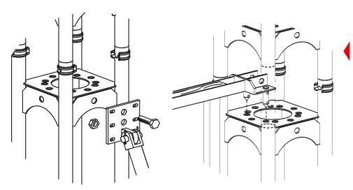
The stiffening bulkhead plates of the frame prop offer many solutions for the connection of scaffold tubes for bracing, working platforms and struts.
